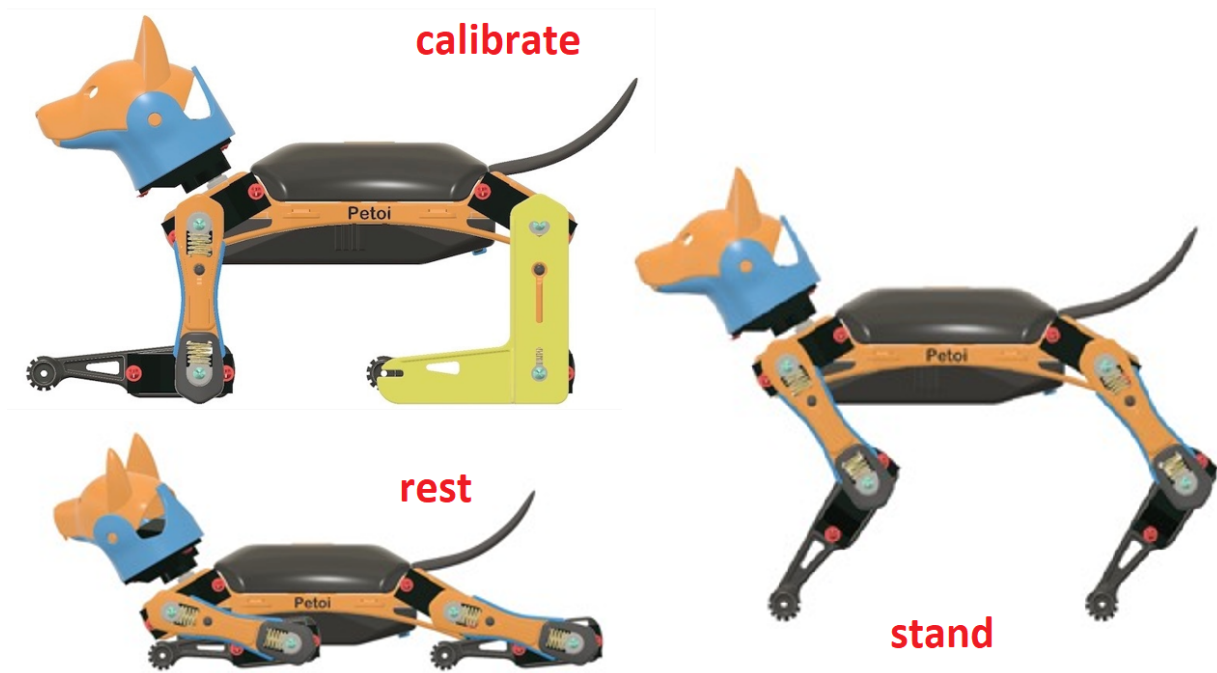
Fig. 8.25: Various postures of Bittle used for calibration.
