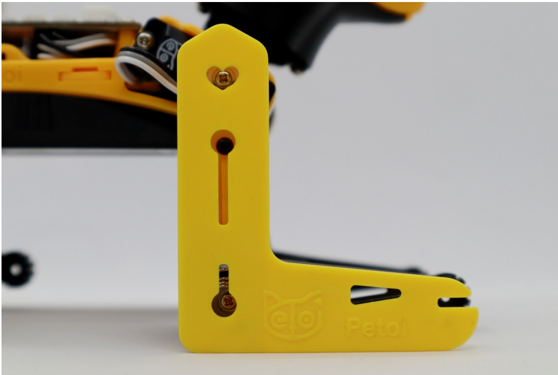
Fig. 8.23: Calibration Tool placement (L tool).
