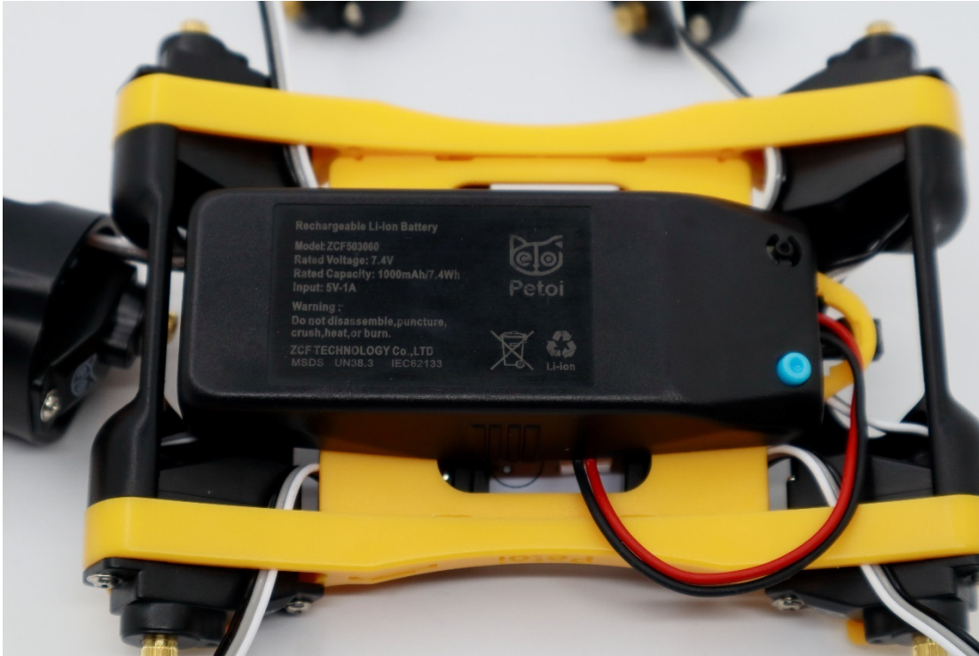
Fig. 8.21: Battery location and status LED.
