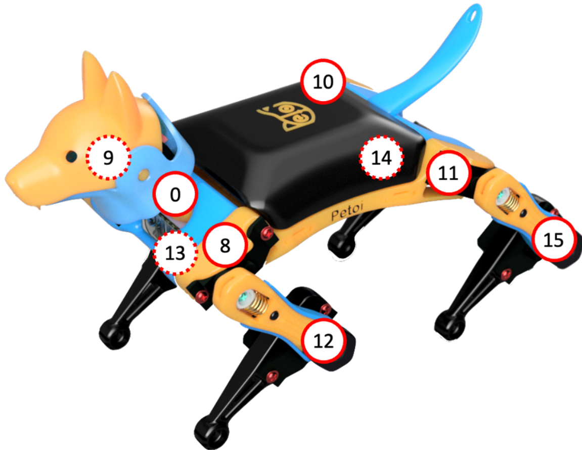
Fig. 8.22: Motor index for calibration.
