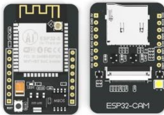
Fig. 8.44: ESP32 Cam Board layout (ref: https://docs.ai-thinker.com/en/esp32-cam )
